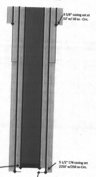
Cement will be Class "C" neat with a slurry volume of 1.32 CuFt/Sk 14.8 Lbs/Gal
