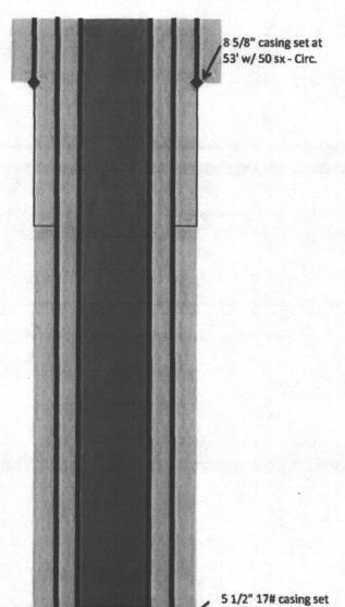
Cement will be Class "C" neat with a slurry volume of 1.32 CuFt/Sk 14.8 Lbs/Gal
