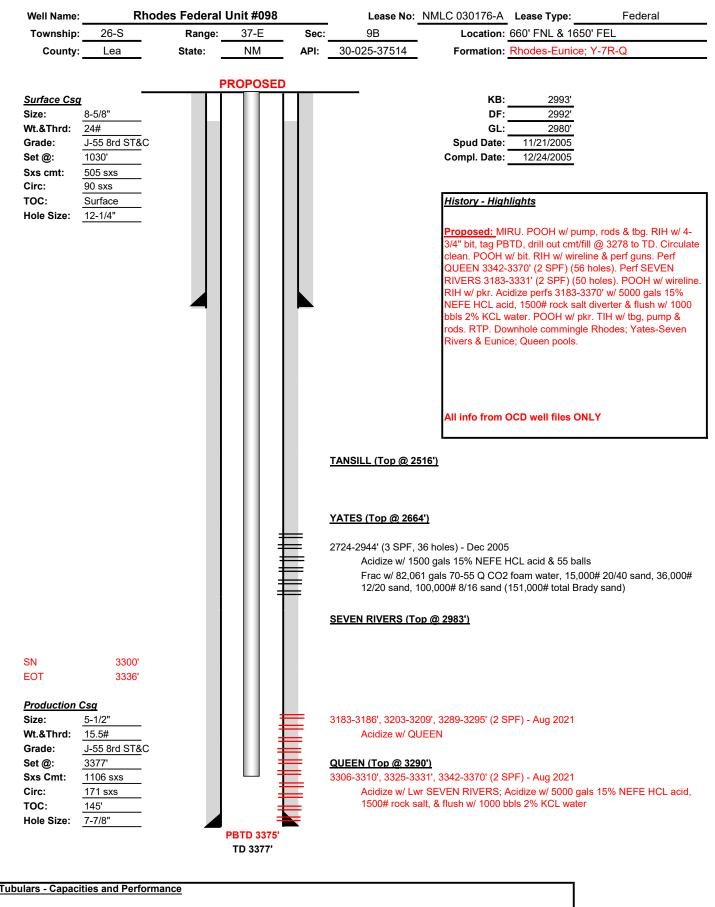
2-3/8" 4.7# EUE 8rd Tubing (~105 jts 2-3/8" tbg, SN, perf sub, MA w/ bull plug) @ 3336'
