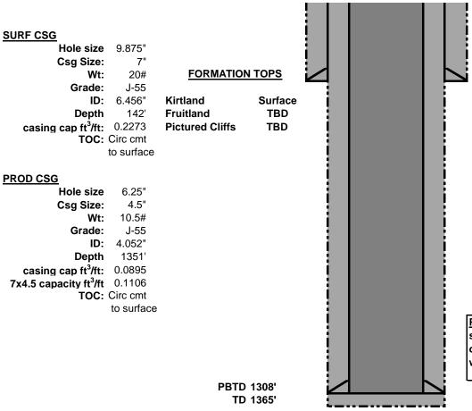
Plug 1: 7/13/21: Mixed and pumped 102 sx cement from 1308' to surface. Topped off cellar with 20 sx. All cement plugs were Class G at 15.8 ppg, 1.15 ft3/sk yield.
