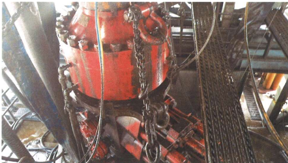
Figure 1: Winch System attached to BOP Stack
