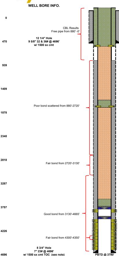
**PLUG #3.** 11-18-21 PUH & PERF'D @ 503'. 11-19-21 EPIR, CIRC WELL W/ 200 SX CLASS "C" CMT. CIRC 7" X 9 5/8" TO SURF. RDMO, **CUT OFF WH, INSTALL DRY HOLE MARKER,** CLEAN LOCATION, P&A COMPLETED 11-19-21.
