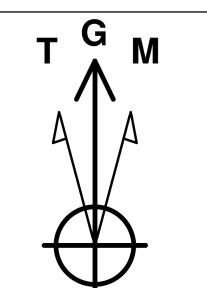
Azimuths to Grid North True North: -0.36° Magnetic North: 6.25°
