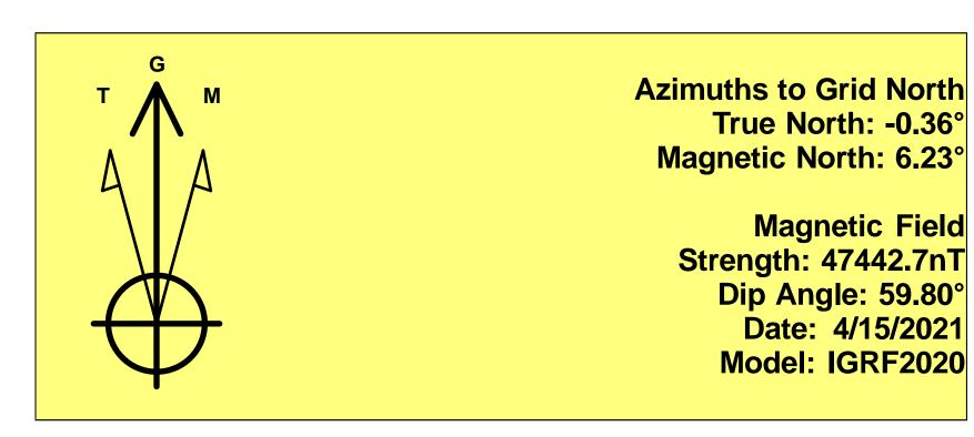
To convert a Magnetic Direction to a Grid Direction, Add 6.23°
