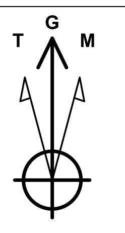
**Azimuths to Grid North** Magnetic North: 6.53° Magnetic Field Strength: 47467.6nT Dip Angle: 59.91° Date: 11/17/2021 Model: IGRF2020
