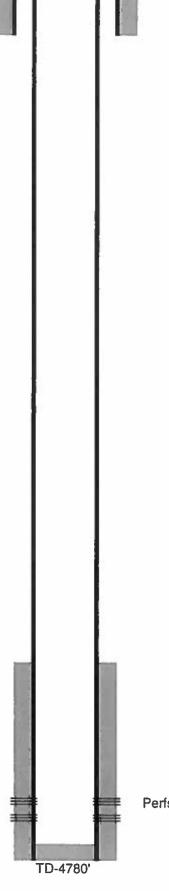
12-1/4" hole @ 303' 8-5/8" csg @ 303' w/ 150sx-TOC-Surf-Circ
