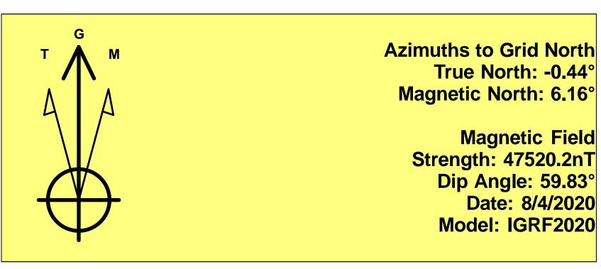
To convert a Magnetic Direction to a Grid Direction, Add 6.16° To convert a Magnetic Direction to a True Direction, Add 6.60° East To convert a True Direction to a Grid Direction, Subtract 0.44°
