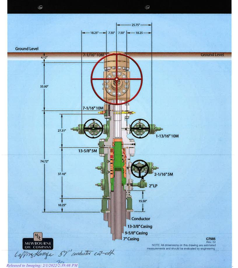
FNR 17/20 W2IP Fed Com #3H Intermediate Casing
