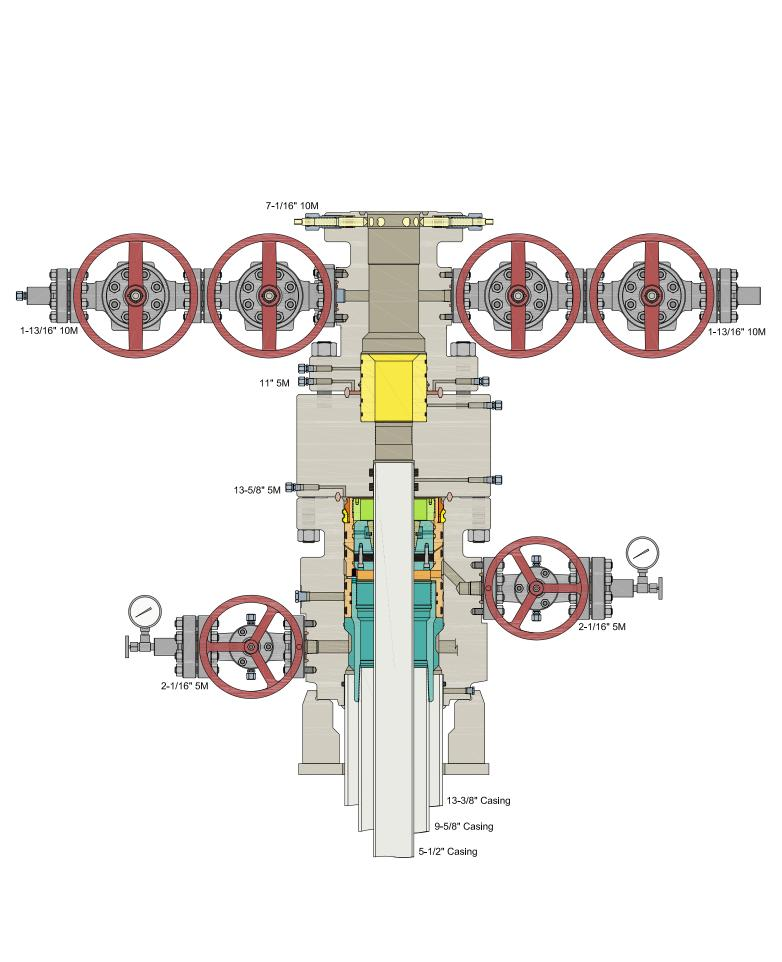
A multibowl wellhead may be used. The BOP will be tested per Onshore Order #2 after installation on the intermediate 1 casing which will cover testing requirements for a maximum of 30 days. If any seal subject to test pressure is broken the system must be tested.
