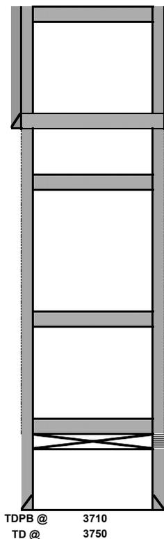
5. Perf'd @ 200'. Pressured up on perfs to 600 PSI. Spotted 25 sx class C cmt @ 250' & circulated to surface.
