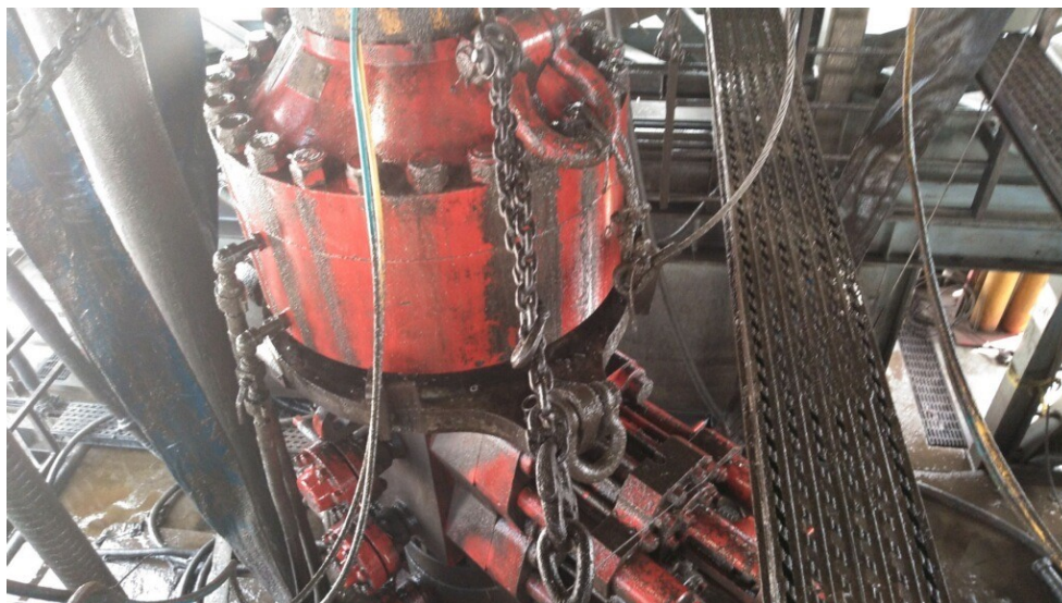
Figure 1: Winch System attached to BOP Stack
