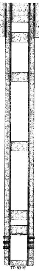
12-1/4" hole @ 1210' 9-5/8" csg @ 1210' w/ 835sx-TOC-Surf-Circ-1"
