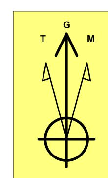
**Azimuths to Grid North** True North: -0.47° Magnetic North: 6.07°
