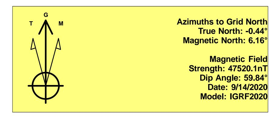
To convert a Magnetic Direction to a Grid Direction, Add 6.16° To convert a Magnetic Direction to a True Direction, Add 6.60° East To convert a True Direction to a Grid Direction, Subtract 0.44°
