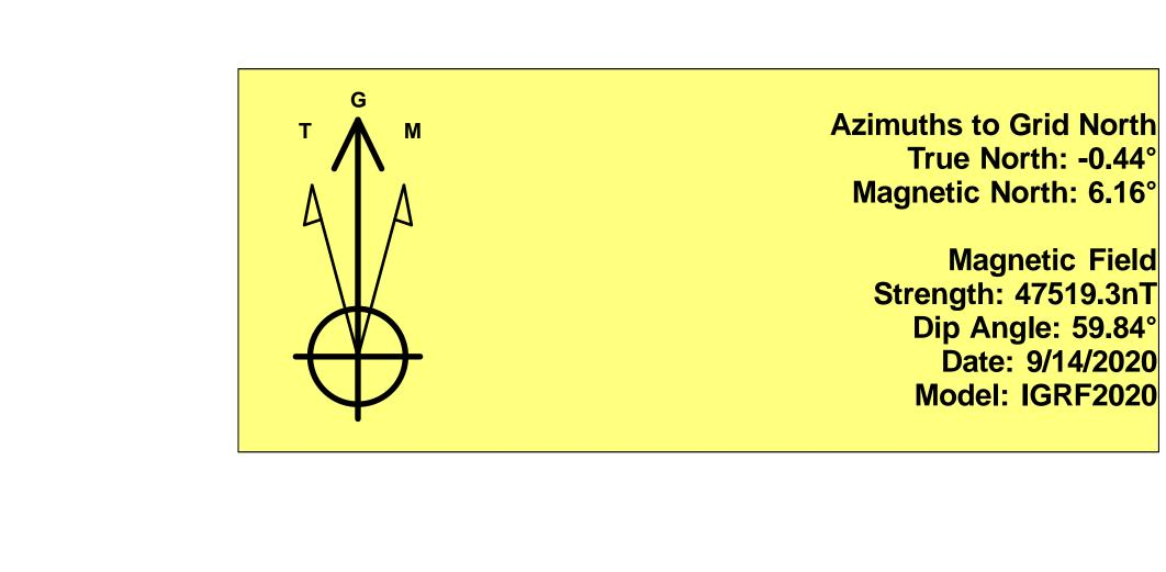
To convert a Magnetic Direction to a Grid Direction, Add 6.16° To convert a Magnetic Direction to a True Direction, Add 6.60° East To convert a True Direction to a Grid Direction, Subtract 0.44°
