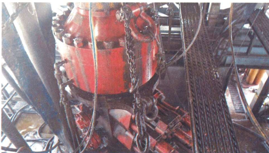
Figure 1: Winch System attached to BOP Stack
