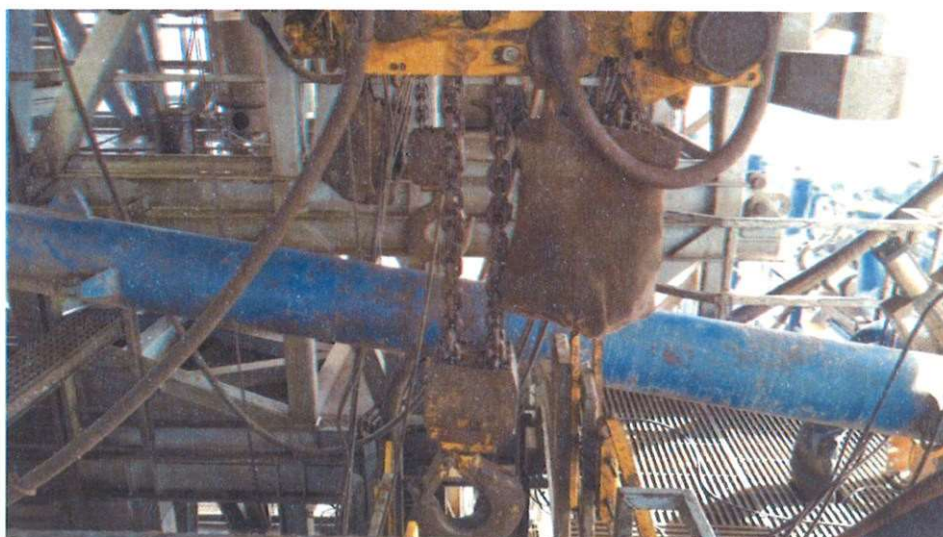
Figure 2: BOP Winch System
