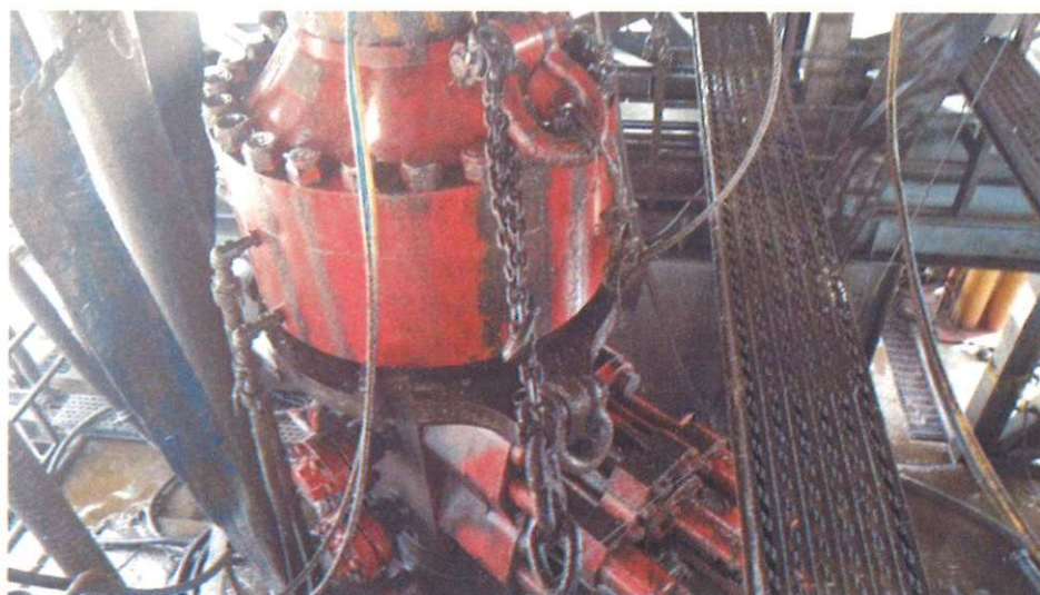
Figure 1: Winch System attached to BOP Stack
