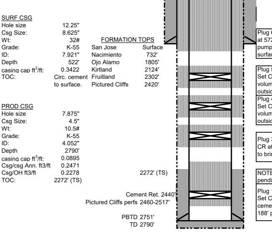
Plug 6: Surface shoe and plug: Perf holes at 572'. Tie onto 4-1/2" casing. Mix and pump sufficient volume to bring cement to surface inside and outside.
