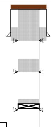
Tubing in well - 2-3/8" tubing Tubing run to 1742'
