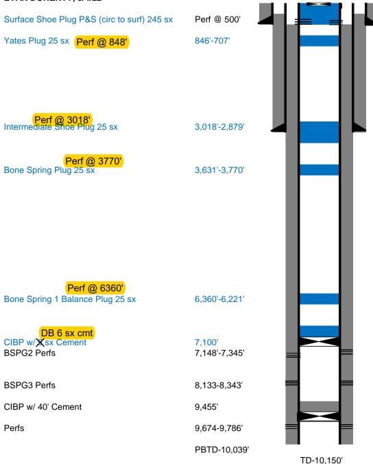
17-1/2" hole @ 450' 13-3/8" csg @ 448' w/ 400sx-TOC-Surf-Circ
