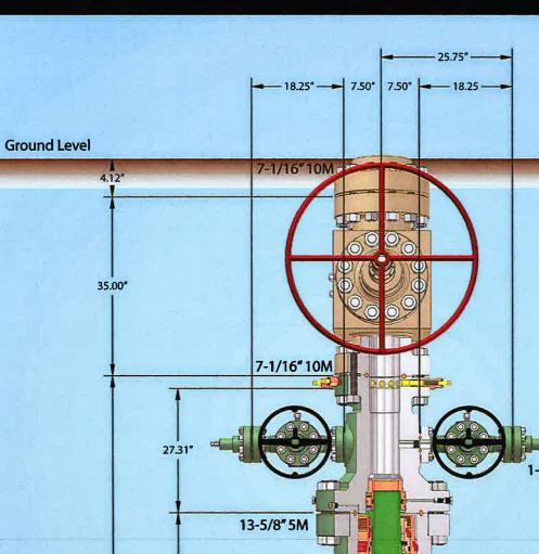
1-13/16" 10M 74.72" 37.16" 2-1/16" 5M 2"LP 15.50" 10.25" Conductor 13-3/8" Casing 9-5/8" Casing 7" Casing C7585 Rev. 02 MEWBOURNE OIL COMPANY NOTE: All dimensions on this drawing are estimated Tirs Hange 57" conductor cut-off measurements and should be evaluated by engineering.
