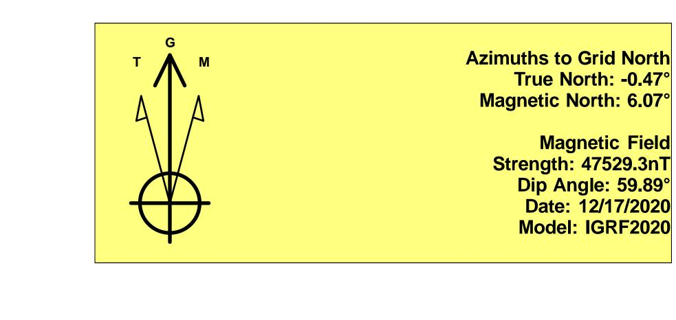
To convert a Magnetic Direction to a Grid Direction, Add 6.07° To convert a Magnetic Direction to a True Direction, Add 6.54° East To convert a True Direction to a Grid Direction, Subtract 0.47°
