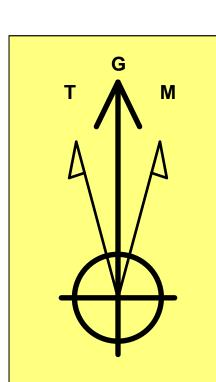
**Azimuths to Grid North** True North: -0.47° Magnetic North: 6.07°
