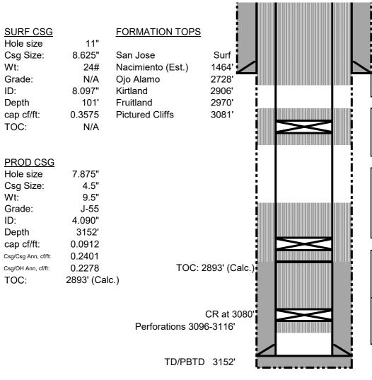
Plug 5: Surface shoe and surface plug: Perf holes at 151'. Tie onto 4-1/2" casing and mix and pump sufficient cement to bring TOC to surface, inside and outside.
