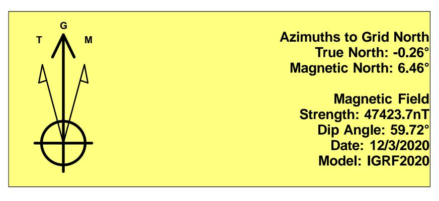
To convert a Magnetic Direction to a Grid Direction, Add 6.46° To convert a Magnetic Direction to a True Direction, Add 6.72° East To convert a True Direction to a Grid Direction, Subtract 0.26°
