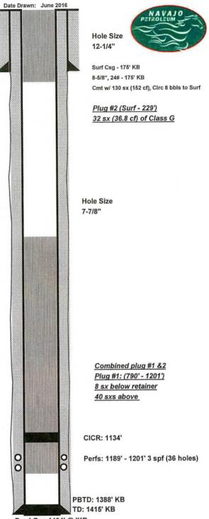
Prod Csg 1404' @ 'KB 38 Joints of 5.5",15.5lb,J55 LT&C CMT: LEAD: 175SX(338cf) , TAIL: 140SX(161cf) CIRC 35BBL CMT to surface
