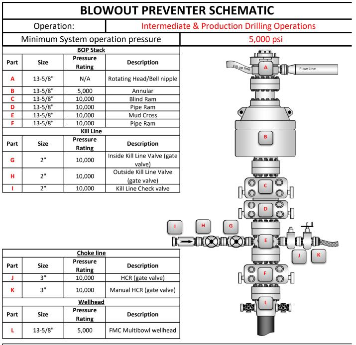
BOP Installation Checklist: The following items must be verified and checked off prior to pressure testing BOP equipment
