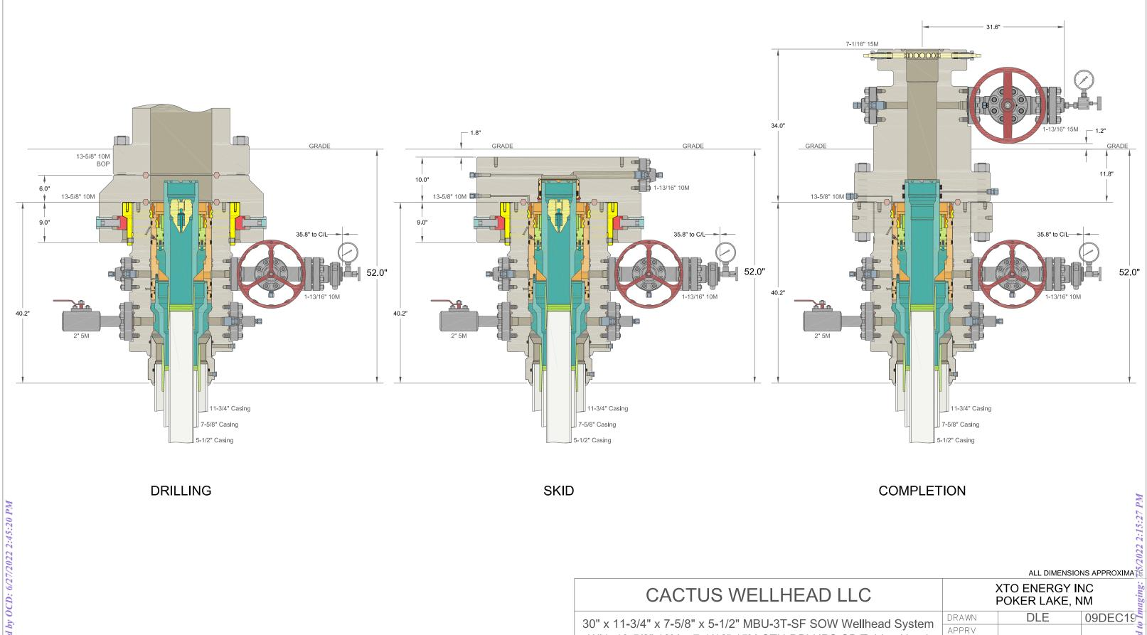
FORMATION CONTAINED HEREIN IS THE PROPERTY OF CACTUS WELLHEAD, LLC. REPRODUCTION, SCLOSURE, OR USE THEREOF IS PERMISSIBLE ONLY AS PROVIDED BY CONTRACT OR AS EXPRESSLY UTHORIZED BY CACTUS WELLHEAD, LLC. 30" x 11-3/4" x 7-5/8" x 5-1/2" MBU-3T-SF SOW Wellhead System With 13-5/8" 10M x 7-1/16" 15M CTH-DBLHPS-SB Tubing Head And 7-5/8" & 5-1/2" Fluted Mandrel Casing Hangers
