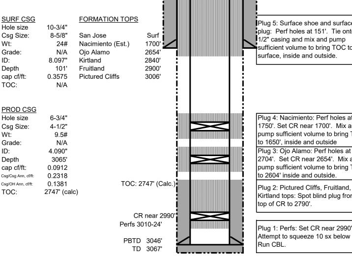
Plug 5: Surface shoe and surface plug: Perf holes at 151'. Tie onto 4-1/2" casing and mix and pump sufficient volume to bring TOC to
