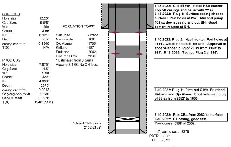
All cement used was Class G mixed at 15.8 ppg, yield 1.15 ft<sup>3</sup> egulatory Representative: Jared Benally, BLM and Monica Kuehling, NMOCD via phor GPS Coordinates: Lat; 36.26482 N, Long; 107.39683 W
