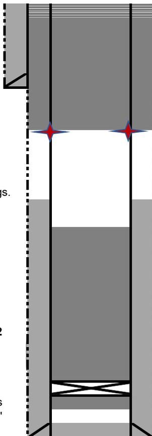
6-8-2022: Cut off WH, install P&A marker, top off casings and cellar with 26 sx.
