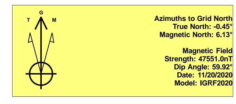
To convert a Magnetic Direction to a Grid Direction, Add 6.13° To convert a Magnetic Direction to a True Direction, Add 6.57° East To convert a True Direction to a Grid Direction, Subtract 0.45°
