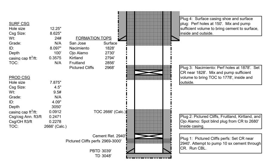
Note: All plugs will include 50' excess cement inside casing, and 100% excess cement outside casing.
