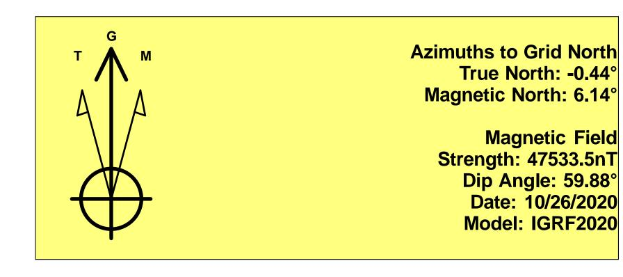
To convert a Magnetic Direction to a Grid Direction, Add 6.14° To convert a Magnetic Direction to a True Direction, Add 6.58° East To convert a True Direction to a Grid Direction, Subtract 0.44°
