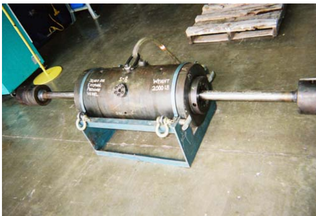
TEST SPECIMENS INSIDE THE EXTERNAL PRESSURE CHAMBER
