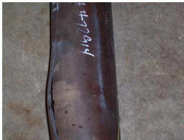
EXAMPLE OF INTERNAL PRESSURE TO FAILURE
