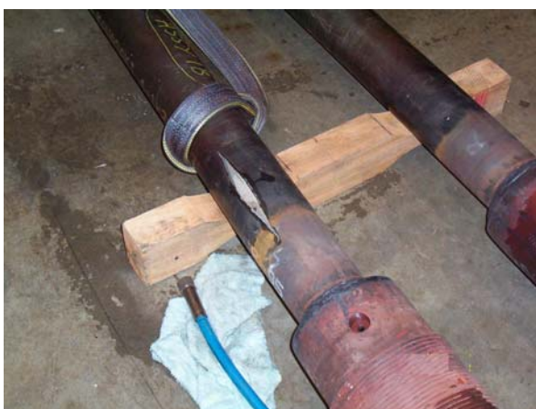
EXAMPLE OF INTERNAL PRESSURE TO FAILURE
