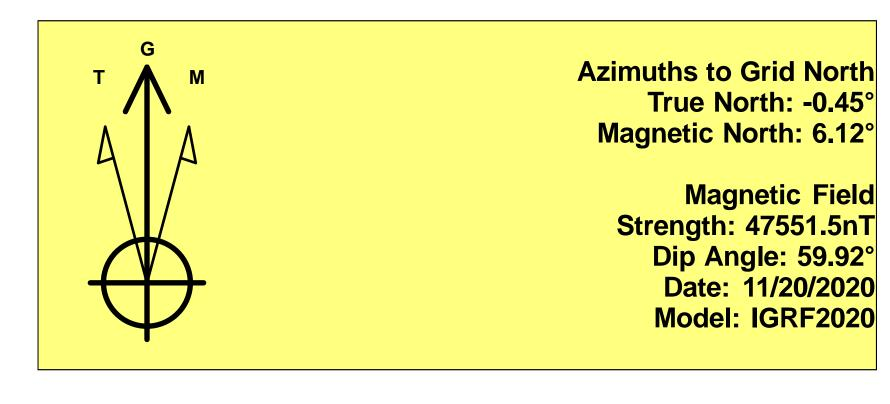
To convert a Magnetic Direction to a Grid Direction, Add 6.12° To convert a Magnetic Direction to a True Direction, Add 6.57° East To convert a True Direction to a Grid Direction, Subtract 0.45°
