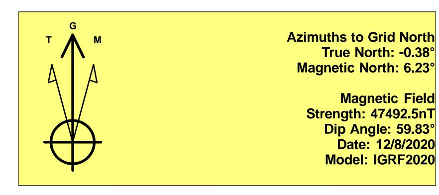
To convert a Magnetic Direction to a Grid Direction, Add 6.23° To convert a Magnetic Direction to a True Direction, Add 6.62° East To convert a True Direction to a Grid Direction, Subtract 0.38°
