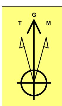
**Azimuths to Grid North** True North: -0.28° Magnetic North: 6.65°
