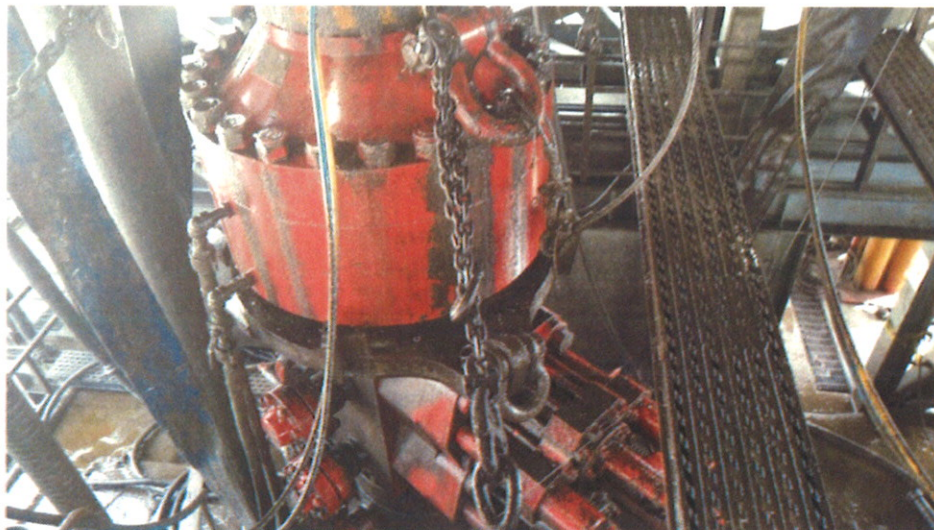
Figure 1: Winch System attached to BOP Stack
