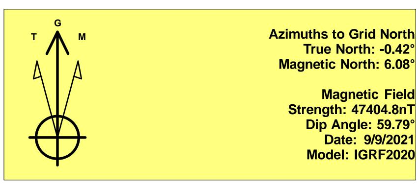
To convert a Magnetic Direction to a Grid Direction, Add 6.08° To convert a Magnetic Direction to a True Direction, Add 6.50° East To convert a True Direction to a Grid Direction, Subtract 0.42°
