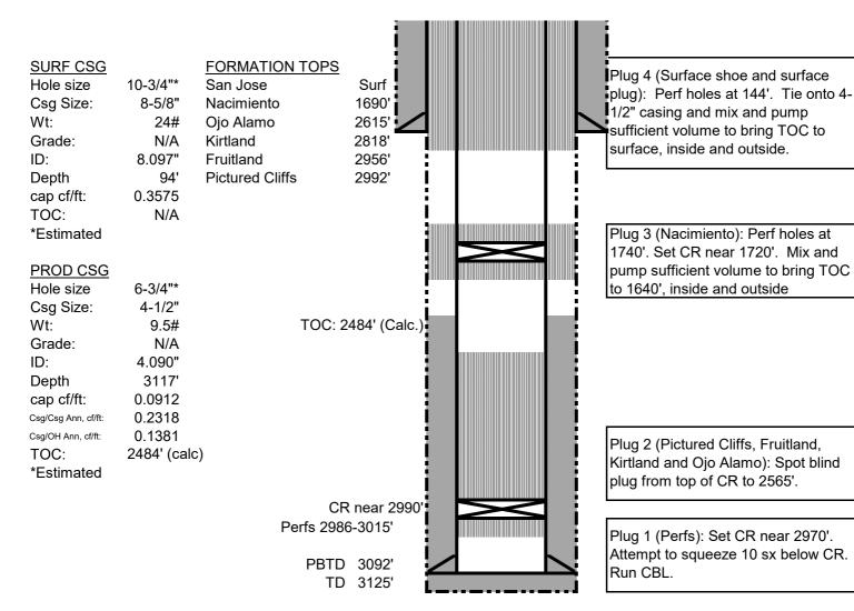
Note: Inside plugs will include 50' excess cement, while outside plugs will include 100% excess
