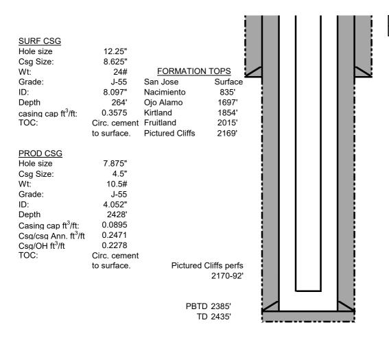
Production Tubing Detail 2-3/8" tubing. EOT 2117'. SN 2083'
