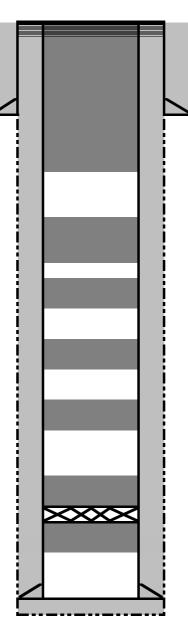
Plug 6: Kirtland and Ojo Alamo tops, surface casing shoe to surface: Spot balanced plug from 614' to surface. Cut off WH, install P&A marker, top off casings and cellar.
