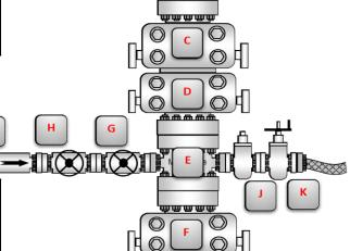
**Choke line Pressure Part** Size Description Rating 3" 10,000 HCR (gate valve) 3" K 10,000 Manual HCR (gate valve) Wellhead Pressure **Part** Size Description Rating
