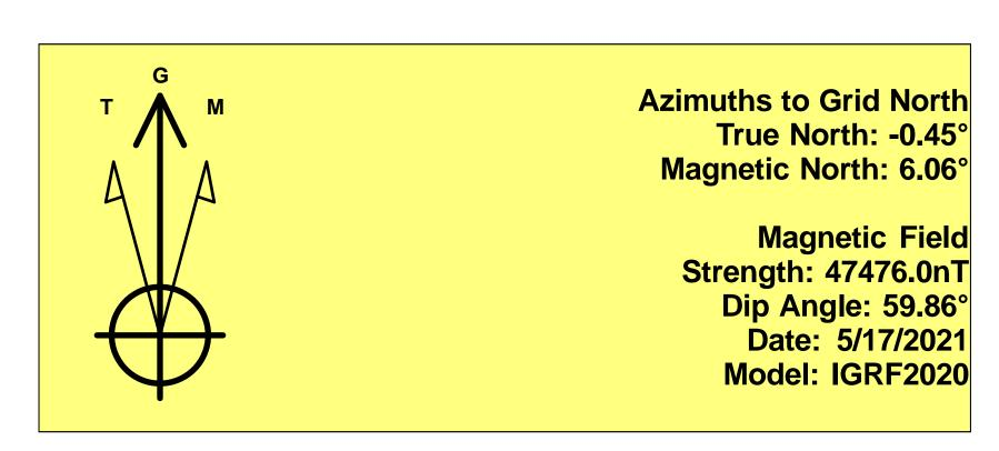
To convert a Magnetic Direction to a Grid Direction, Add 6.06° To convert a Magnetic Direction to a True Direction, Add 6.51° East To convert a True Direction to a Grid Direction, Subtract 0.45°
