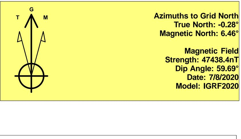
To convert a Magnetic Direction to a Grid Direction, Add 6.46° To convert a Magnetic Direction to a True Direction, Add 6.74° East To convert a True Direction to a Grid Direction, Subtract 0.28°
