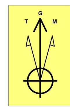
**Azimuths to Grid North** True North: -0.28° Magnetic North: 6.47°
